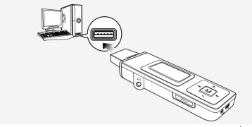
Remove the USB Cover then connect the USB Connection Plug to the USB port (  $\psi$  ) on your PC.
